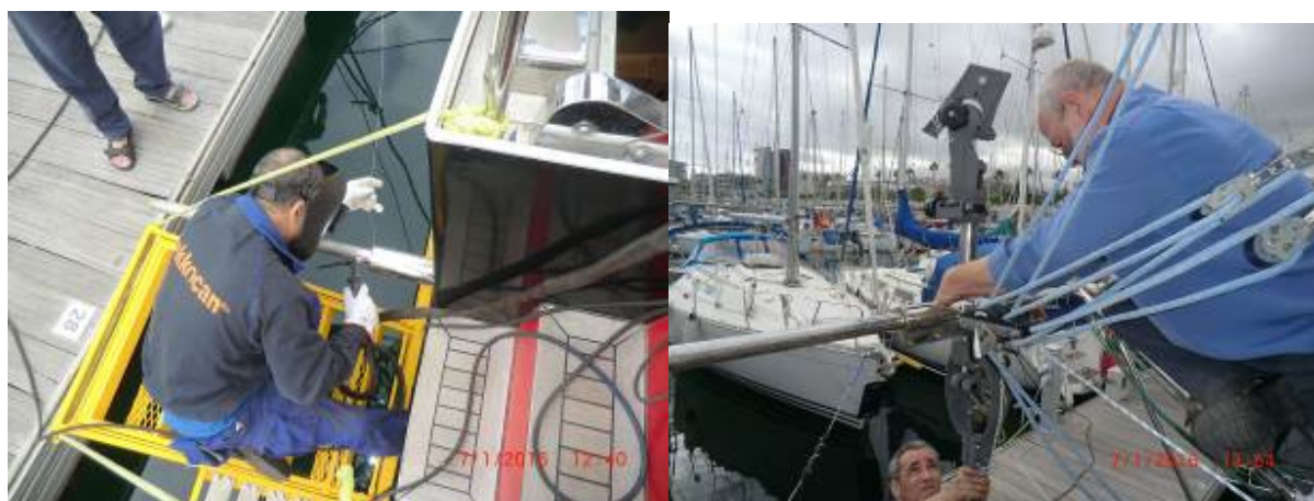
Aligning the Hydrovane in the vertical, using high tech: a piece of cord with heavy screws at the end.
